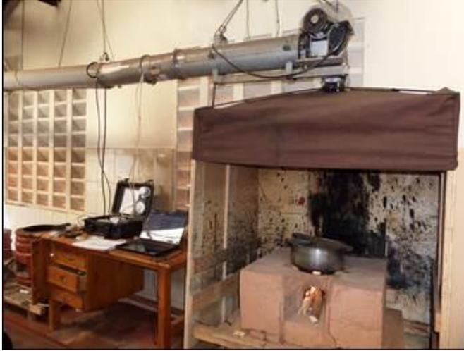
Figure 2: Canarumwe stove under the PEMS hood for WBT, Emissions and indoor emissions test.
